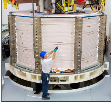
One of the seven central solenoid modules GA is supplying to ITER
